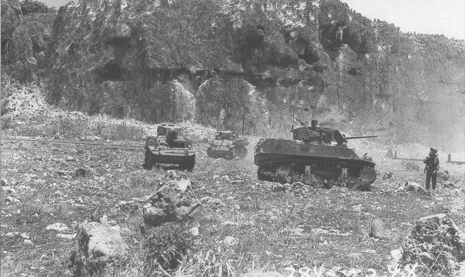
"Nannie", a M5A1 light tank of Co. D, 4th Marine Tank Battalion, escorts a M3A1 Satan flamethrower tank during the fighting against Japanese infantry holed up in caves in the cliffs at Marpi Point. Flamethrower tanks were usually accompanied by normal gun tanks to provide protection. By this stage in the war, the anti-personnel cannister round had become one of the M5A1s main weapons, due to the lack of Japanese tanks.
