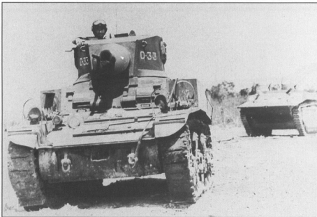
A M3A1 Satan flamethrower tank escorts a LVT-3 amtrac during the fighting near Tanapag, Saipan on 7 July 1944. Notice that the front hull machine gun of the flamethrower tank was blanked off since this was removed to provide needed storage.
