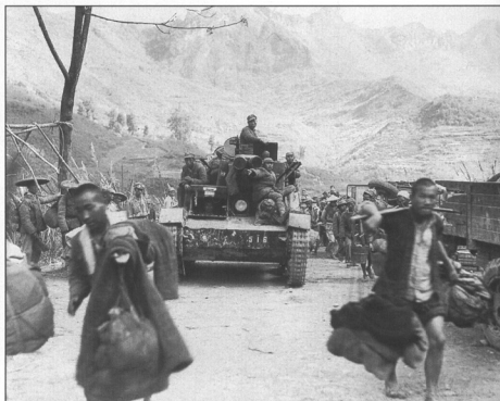
A Chinese T-26 Model 1933 moves along the road at the time of the Japanese offensive in November 1944 near Chin Chen-chaing China. This vehicle shows the location of the standard tactical markings on the tank bow. Notice also that this vehicle is fully equipped with searchlights over the gun barrel.
