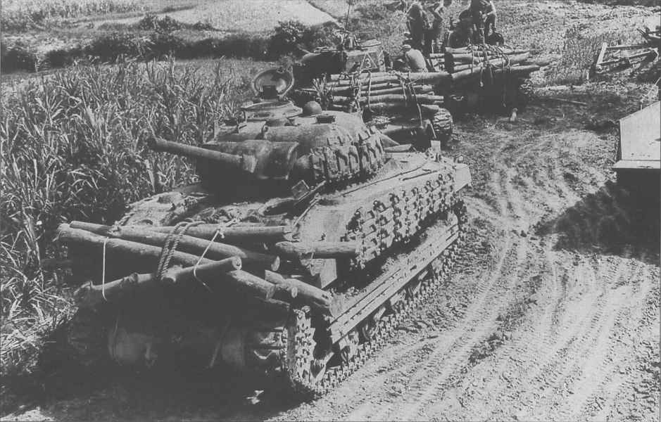
A M4A2 (W) medium tank of the 1st Marine Tank Battalion on Okinawa loaded with timbers. These were used to fill Japanese anti-tank ditches. Japanese engineers often created elaborate tank traps in front of defensive positions to hinder tanks and force them into killing zones covered by anti-tank guns or mines. This also gives a good impression of the extensive applique armor added to Marine tanks by the time of the Okinawa fighting.
