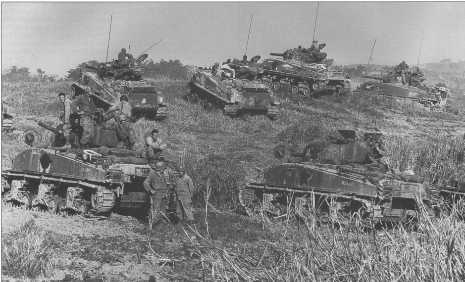
Composite hull M4 "blow-torch" medium tanks and M4 105mm howitzer tanks of the 713th (Flamethrower) Tank Battalion take up positions along a ridge line during the landings on Okinawa in April 1945. The tanks in the foreground are flamethrower tanks. The 105mm howitzer tanks are new production vehicles with HVSS suspension. These vehicles were used by the headquarters company in tank battalions to provide fire support. Many of the vehicles have improvised camouflage, and all have their white identification stars painted out. By this stage of the war, most Japanese infantry regiments had been equipped with 47mm anti-tank guns, which were very effective against the M4 medium tank at the usual battle ranges in the Pacific theatre.
