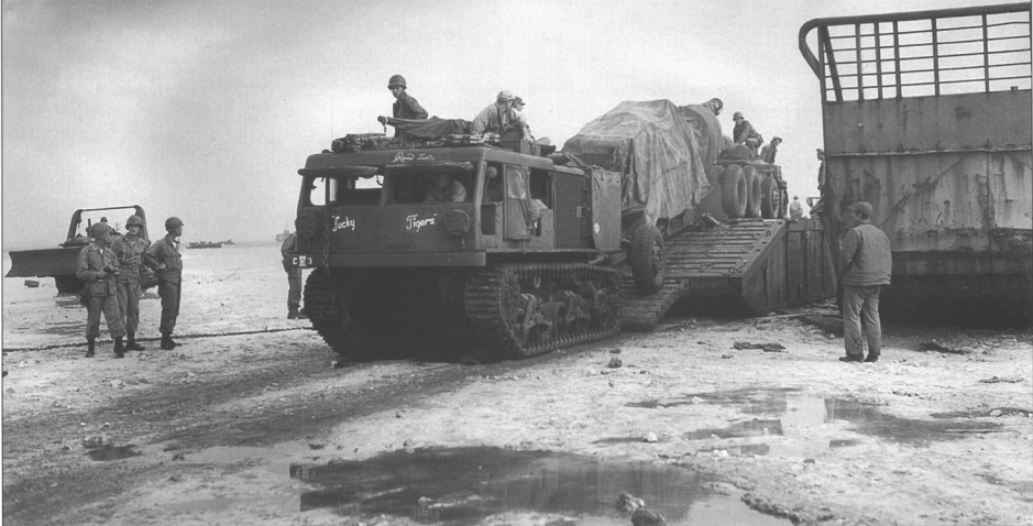
The largest amphibious operation in 1945 was the assault on Okinawa. This is a M4 18-ton high speed tractor towing a 155mm "Long Tom" gun off a landing pier at Keise Shima on 31 March 1945, the day before the main landing. The artillery was deployed on Keise Shima to conduct artillery bombardment prior to the main landing.
