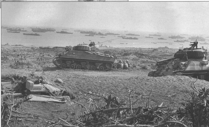
With the experiences of previous campaigns, Marine tank deployed on Iwo Jima in February 1945 were well prepared to deal with Japanese infantry anti-tank tactics. This M4A2 (W) of the Marine 5th Tank Battalion has planking on the side to prevent the attachment of magnetic mines, and penny nails welded to the turret hatches to prevent the attachment of satchel charges intended to blow open the hatches. This tank became bogged down near the landing beaches in the soft volcanic soil.
