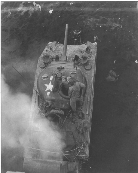
M4A2 (W) medium tanks of the 5th Marine Tank Battalion in a bivouac area on 24 February 1945 on Iwo Jima. This shows the characteristic pennynail protection on the hatches used by this battalion, as well as the camouflage painting over the side plating. Many Marine tanks on Iwo Jima had a pattern of sand and red brown painted over the normal olive drab.
