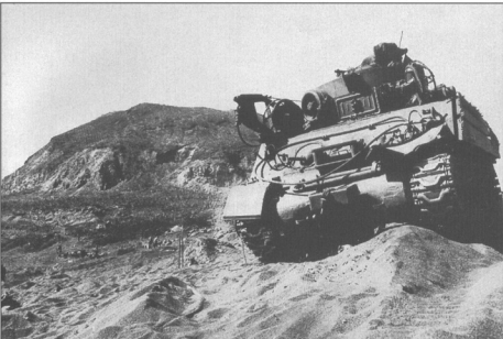
An M32 armored recovery vehicle in the foothills of Mount Suribachi. The soft volcanic soil of the island meant that these vehicles were often put to good use. The American flag raised on Mount Suribachi can barely be seen in this view.
