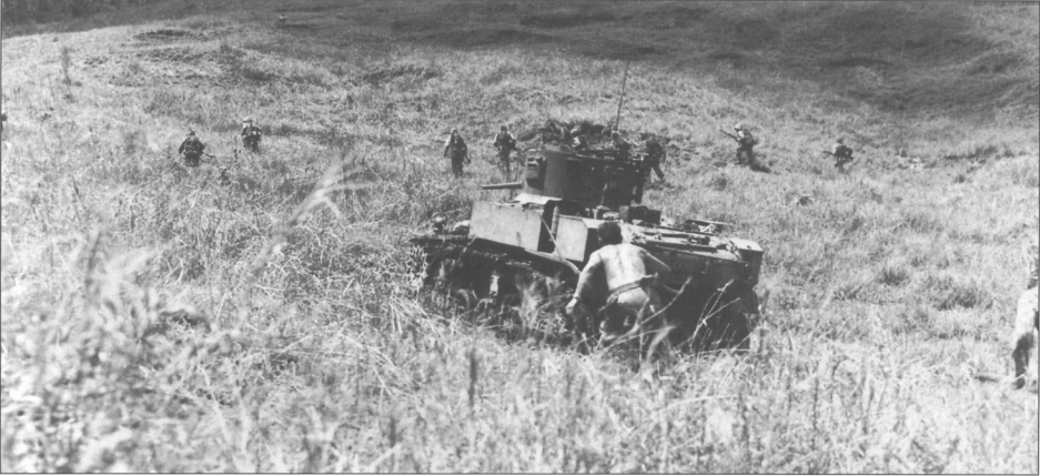
A M3A1 light tank provides fire support for advancing Marines on New Georgia in the autumn of 1943. By this time, the M3 light tank was widely regarded as obsolete, as its 37mm gun was not well suited to attacking Japanese bunkers, one of the main objectives of many tank missions. Indeed, some Japanese bunkers were so thickly constructed that the tanks were forced to actually drive up to the firing slits and fire directly into the bunkers. With the advent of the new Japanese 47mm anti-tank gun, this became impossible.
