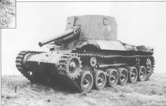
A rear view of a Type 1 Ho-ni 75mm self-propelled gun that was captured by the US Army's 37th Infantry Division near Aritao on 6 April 1945. This vehicle later was sent back for evaluation to Aberdeen Proving Ground, and now rests in the Ordnance Museum there. The white circle insignia surrounding a red circled rectangle was the company insignia of the unit equipped with the Ho-ni.
