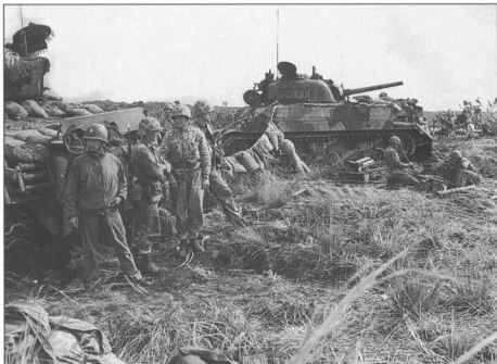
M4A2 (W) medium tanks of the 5th Marine Tank Battalion in a bivouac area on 24 February 1945 on Iwo Jima. This shows the characteristic pennynail protection on the hatches used by this battalion, as well as the camouflage painting over the side plating. Many Marine tanks on Iwo Jima had a pattern of sand and red brown painted over the normal olive drab.
