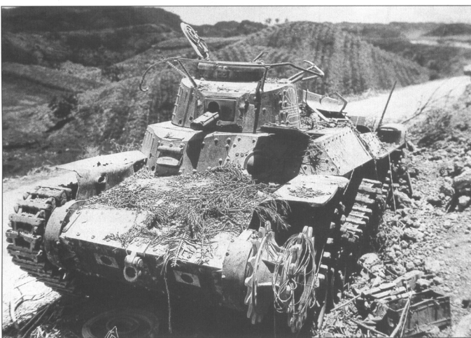
About six Type 97 Chi-ha survived the night attack of the 9th Tank Regiment. This tank of the 5th Company was later knocked out, probably by M5A1 light tanks of the 762nd Tank Battalion. The 57mm gun on this vehicle is missing, and two 37mm hits can be seen immediately below and to the left of the gun mantlet. This view shows the markings of this company: two Japanese flags on the lower bow, and the intricate kikusui emblem on the turret side.
