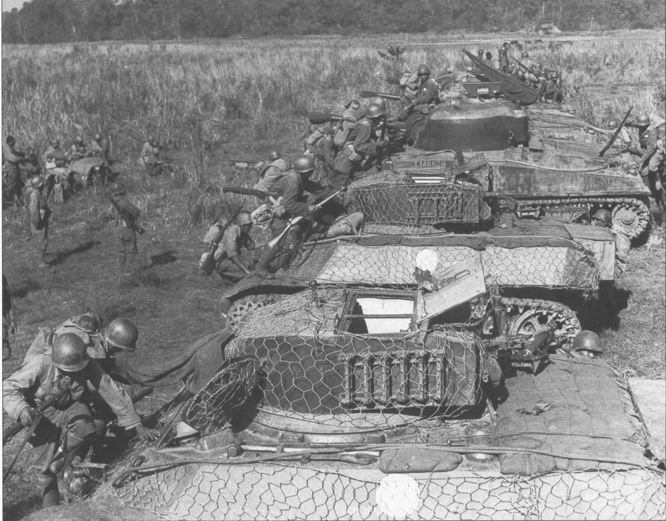
The Chinese 1st Provisional Tank Group was committed to action near Kabani, Burma in January 1945. Here, infantry from the 5332nd Brigade climb on board M4A4 Sherman and M3A3 Stuart tanks. The M3A3 Stuarts are heavily covered in chicken wire to attach foliage for camouflage.
