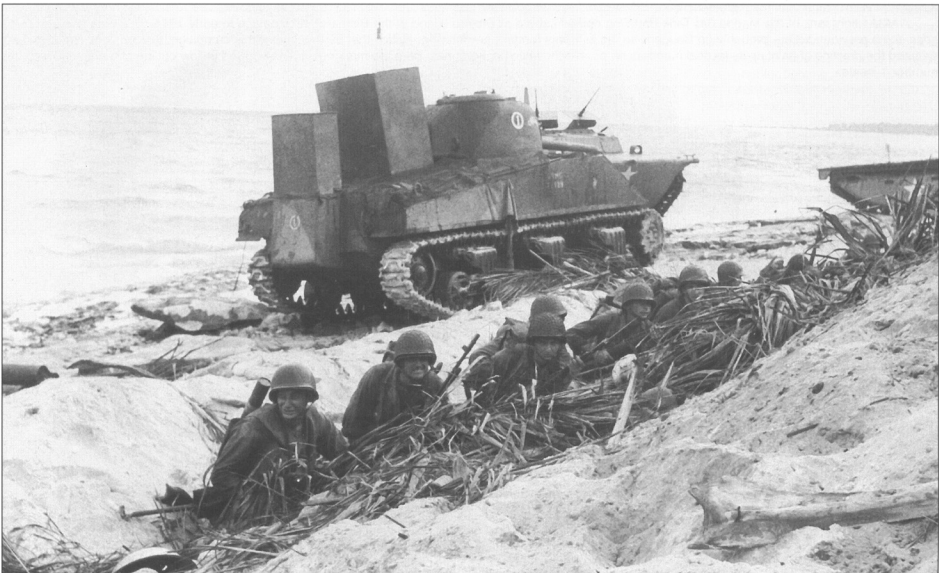
An M4A2 medium tank of the Marine 2nd Separate Tank Company waits along the beach on Perry Island in the Marshalls during the landings there in February 1944. At this stage of the war, the fording trunks were often built by local ordnance teams, and so their shape and configuration differed considerably from the later standardized types.
