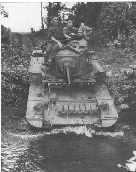
A rare view of one of the few Japanese tanks to fight on American soil in World War 2. This Type 95 Ha-go light tank took part in the fighting on Kiska in the Aleutian island chain off Alaska. A handful of these light tanks were landed on Kiska and Attu in June 1942 when the Japanese Army made unopposed landings, but they saw little action in August 1943 when the US Army landed to retake the islands.
