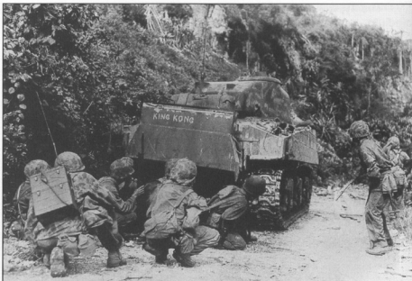
A M4A2 named "King Kong" of Co. C, 4th Marine Tank Battalion supports Marines during the fighting near Marpi Point on 8 July 1944. Many of the crews did not bother to remove the rear wading trunk, although the upper deck trunk was normally removed since it interfered with the traverse of the turret. This tank has the planks on the side typical of this battalion on Saipan, and also has an irregular camouflage pattern, probably applied with mud, on the turret and hull sides.
