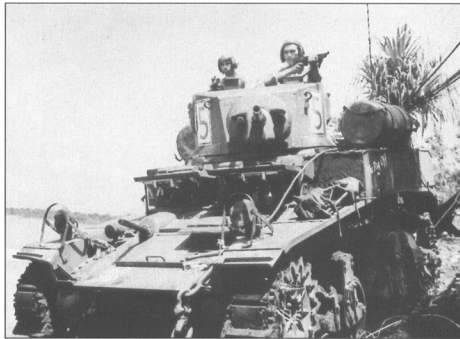
"The Pay-Off", a Marine M3A1 light tank, poses for the camera after landing on Bouganville in the Solomons on 14 November 1943. The two large drums on the rear carry additional fuel. These would usually be dropped before going into combat due to the fire hazard they posed.
