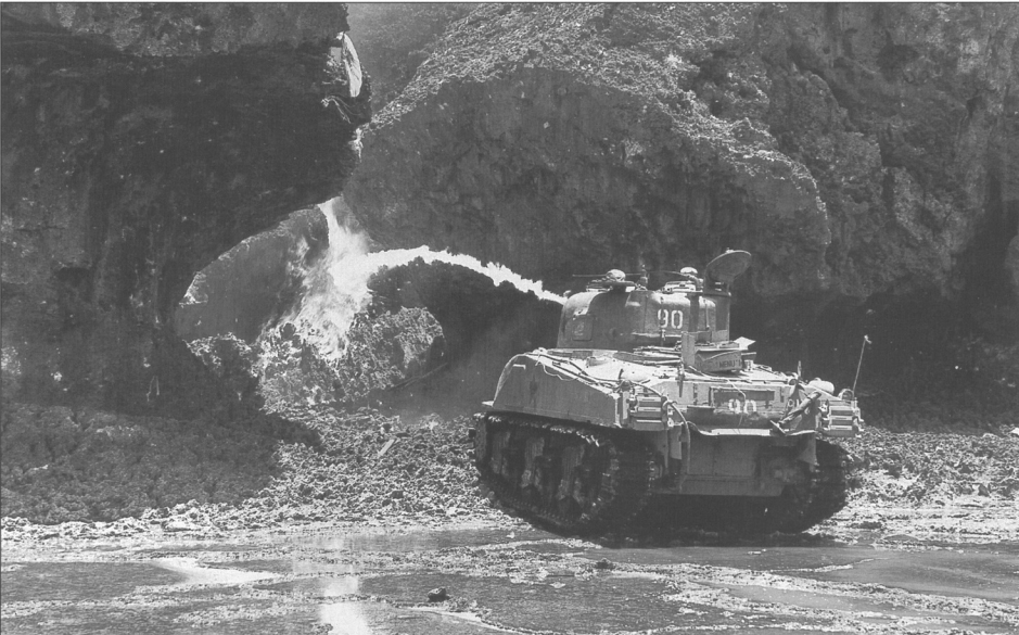
A composite hull M4 Blow Torch of the 713th Flamethrower Tank Battalion attacks Japanese infantry hidden in caves on the southern shores of the island. The fighting on Okinawa, the first fought on Japanese soil, was particularly bitter, and often the local civilians joined the soldiers in the cave.
