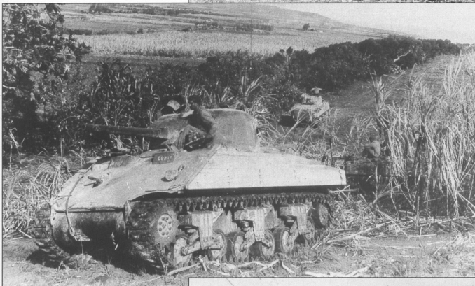
A M4A2 named "Jenny Lee" of the Marine 4th Tank Brigade moves forward on Saipan in July 1944 near Magicienne Bay. This shows the widespread use of wooden planking on the hull side as a form of protection against hand-emplaced Japanese magnetic anti-tank mines, an American equivalent of German zimmerit. Notice also that the tank has a thin coating of concrete applied over the glacis plate, rather than wood, for the same purpose.
