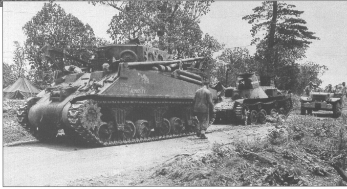
A Type 95 Ha-go light tank, is recovered by a M32 armored recovery vehicle of the Marine 3rd Tank Battalion. It is named "Almighty" and carries the elephant insignia of the 3rd Tank Battalion.
