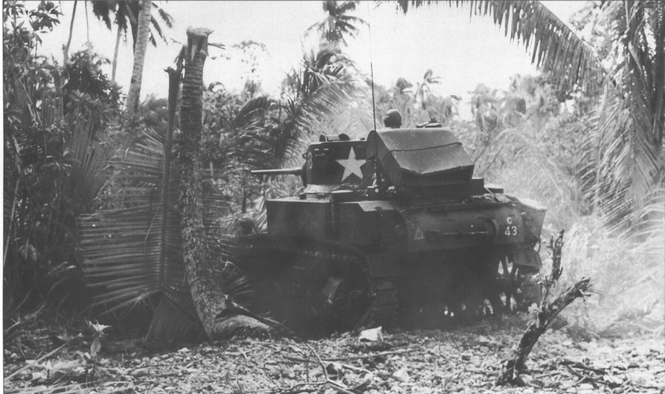
The 193rd Tank Battalion taking part in the Makin operation also had a company of M3A1 light tanks. This M3A1 is moving forward near Red Beach in front of the 165th Infantry to eliminate Japanese snipers on 20 November 1943 shortly after the initial landings on Butaritari. The tank still has its fording trunk on the engine deck.
