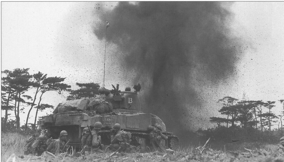
A composite hull M4 medium tank, possibly a flamethrower from the 713th Tank Battalion, comes under fire from Japanese artillery while supporting the 382nd Infantry during fighting on Okinawa on 4 June 1945. Notice the telephone box added on the far left side of the hull rear, a vital new addition to help in tank-infantry coordination.
