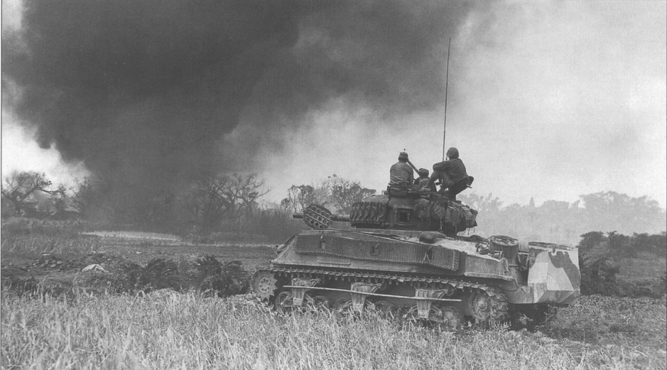
A M4A2 (W) medium tank of the 1st Marine Tank Battalion during fighting on Okinawa in April 1945. The tank still has its deep wading tank attached. The material on the side is apparently intended to offer protection, but it is not clear what type of material it is made from. Normally, Marine tanks used either spare track blocks or wooden planking.
