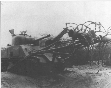
There was less development of specialized armor in the Pacific theatre than in Europe. This is a mine flail developed by US Navy Seabee engineers, however it was never used in combat. Although mines were often a problem during operations, there was no confidence that such flails were practical.
