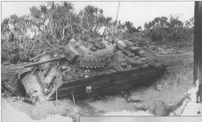
There was less development of specialized armor in the Pacific theatre than in Europe. This is a mine flail developed by US Navy Seabee engineers, however it was never used in combat. Although mines were often a problem during operations, there was no confidence that such flails were practical.
