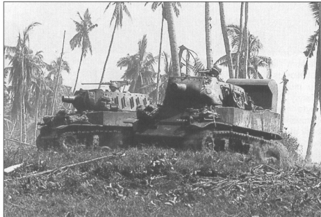
A pair of M8 75mm howitzer motor carriages support the 1st Cavalry Division on Leyte shortly after the landings. The M8 HMCs still have their deep wading stacks attached.
