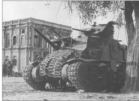
The M3 Lee medium tanks were quickly adapted to the local surroundings like this vehicle of the 150th Regiment RAC during fighting by Major Campbell's C Squadron in Mandalay in February 1945. The spare track was added to the front as expedient armor against Japanese anti-tank guns. During the Mandalay fighting, one Lee was hit no fewer than 13 times by 37mm anti-tank gun fire, yet still remained in action. (IWM)
