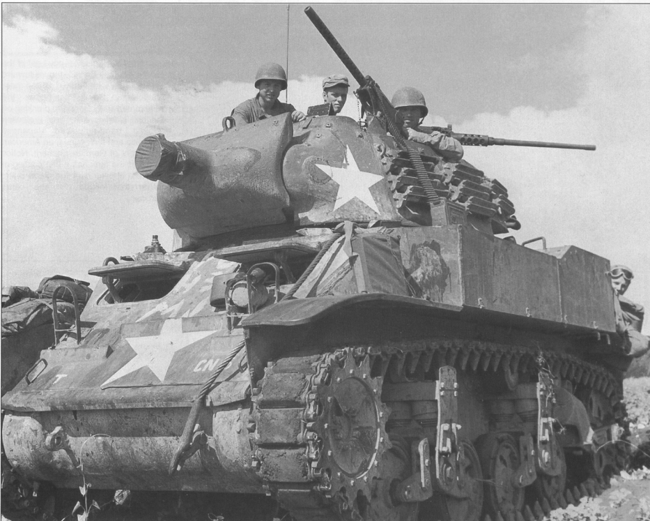
An Army M8 75mm howitzer motor carriage during operations on Saipan. This was based on the M5 light tank chassis, but with a new open-top turret. There were six of these assigned to each armored cavalry squadron, providing fire support to other vehicles in the unit with their short-barreled 75mm howitzer.
