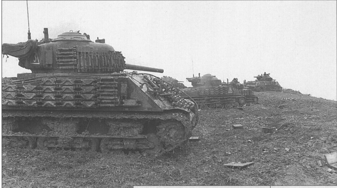
A Marine M4A2 (W) medium tank of the 1st Marine Tank Battalion on Okinawa. This is one of the late production types with the new commander's all round vision cupola. This unit painted its tactical insignia on the upper edge of the turret due to the use of extensive track blocks, in this case a circled number 1.
