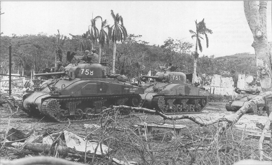
A platoon of composite hull M4 medium tanks of Co. C, 706th Tank Battalion during operations near Agana on Guam on 2 August 1944. The Guam operation followed the Saipan landings. The composite hull M4 was similar to the basic M4 medium tank, but the hull front was a single casting rather than being constructed of the usual welded plates.
