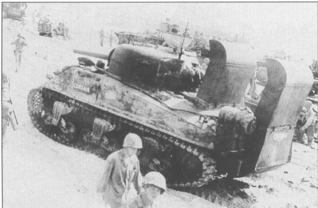
"Corsair", a M4A2 (W) of Co. C, 2nd Marine Tank Battalion, comes ashore at Tinian on 25 July 1944. Tinian was the third of the major islands in the Marshalls attacked by the US forces in July 1944. The Marshalls campaign saw the combat introduction of the late production M4A2 medium tank with the revised 47 degree hull front and wet ammunition storage. By this stage, the deep fording trunks are becoming more standardized than during previous landing operations. This particular tank appears to have a rough coat of camouflage applied over the hull, possibly with mud.
