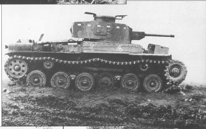
The Saipan campaign was the first encounter where the new Type 97-kai Shinhoto Chi-ha was encountered in significant numbers. Although first deployed in early 1942, the low priority assigned to Japanese tank production meant that few were available in the Central Pacific until 1944. The tank's new 47mm made it capable of defeating the M4 Sherman under the right circumstances. This is a tank of the regimental command platoon, evident from the white band markings around the turret.
