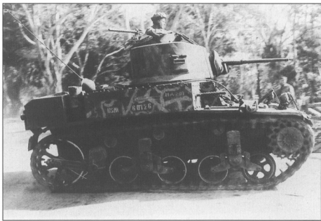
A M3 light tank of the US Marine Corps 1st Tank Battalion during training prior to the Solomons campaign in November 1942 in New Zealand. This M3 light tank is from the later production batches with the round turret and the added rear storage bins. Notice also that the tank commander wears the early pattern US tanker's helmet with the thick leather band around the rim.
