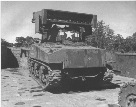
There were a number of experimental rocket launchers tested in the Pacific theatre as a potential source of fire support. This M4A2 medium tank named "Detour" is fitted with the 7.2 inch M17 "Whizbang" rocket launcher. So far as is known, none of these were actually used in combat in the Pacific.
