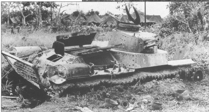
A Type 97 Chi-ha of the 4th Company, 9th Tank Regiment that became bogged down in soft soil during the 16 June attack. Notice that a frame has been attached at the rear of the tank. This was added on many tanks to permit them to carry infantry along during the attack.
