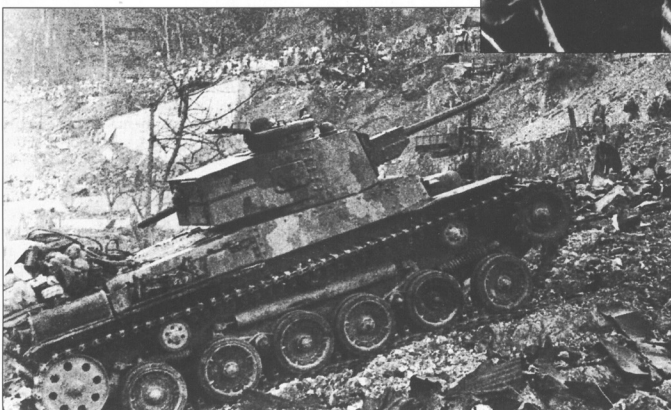
The assault on Corregidor was the combat debut of the Type 97-kai Shinhoto Chi-ha medium tank. This version of the tank substituted the new 47mm gun for the earlier short 57mm which was not very effective when facing enemy armor. The tank detachment from the 7th Tank Regiment that landed on Corregidor consisted of two of these tanks, plus a captured US Army M3 light tank commanded by Maj. Matsuoka.
